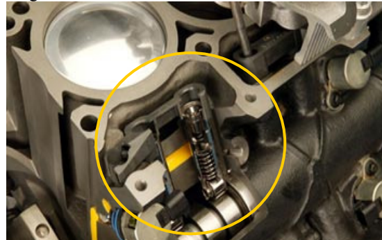
Slika 1 - Multy-Displacement System (MDS)
