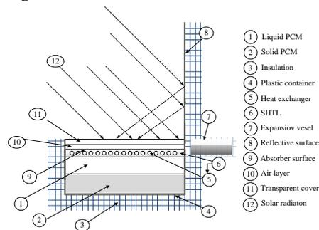
Figure.3 – Integrated PCM solar collector storage system designed
