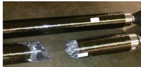
*Figure 1- Fracture of one-piece composite drive shaft*
