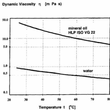
*Figure 3. Viscosity of water and mineral hydraulic oil*
