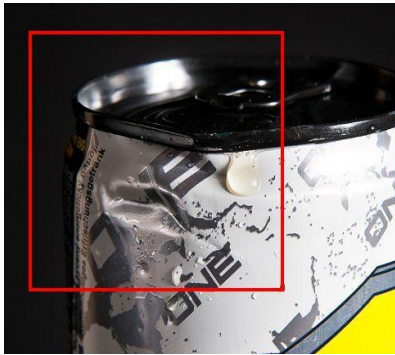
Figure 1 - Mechanically damaged can
